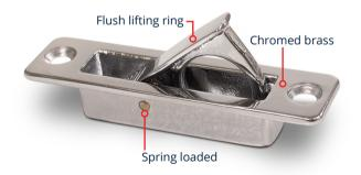
The PYI Floor Latch is made of chromed brass. It features a flush lifting ring, and when pressed the latch opens due to the loaded spring.
