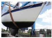
Boat hull after being in the water for 2 years with the Sonihull system.
