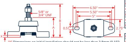
"X" Dimensions on initial installation should not be less than 3.8mm (0.15").
