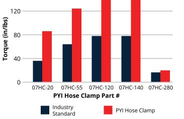
\*\* The Destructive Torque Test measures how much force is required to break the hose clamp (higher is better).
