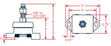
"X" Dimensions on initial installation should not be less than 3.8mm (0.15").
