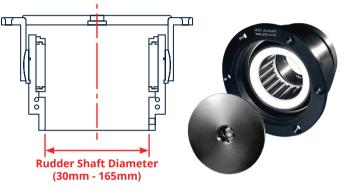
emergency tiller arrangement type 1, a quick and safe access to the emergency steering is achieved. The bearing is available in specific sizes, so take notice when designing the rudder stock.
