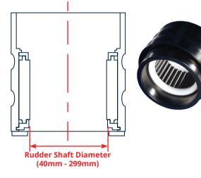
The bearing can be sealed by a rudder tube or double lip seal inside the top register of the inner housing, or for maximum security a rudder tube in the top register in the outer housing.
