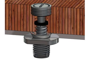
PYI "OEM" Floor Anchors are designed to allow a ¾" (9mm) to ¾" (19mm) floor panel to be attached and detached repeatedly. PYI "OEM" Floor Anchors are a simplified form of PYI's successful Floor Anchors. Their simple design and installation allows a production boat builder to implement this type of fastener in a manufacturing environment. All components are made from 304 stainless steel.
