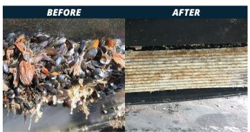
One years growth <u>without</u> Sonihull After one year <u>with</u> Sonihull Ultrasonic Antifouling. Ultrasonic Antifouling system.
